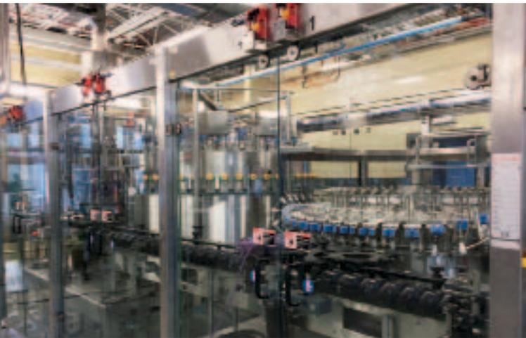
*The new state-of-the-art brewing facility features upgraded equipment, such as a new centrifuge and packaging line. The computer-run system is more efficient, reduces loss and maintains consistency.*
